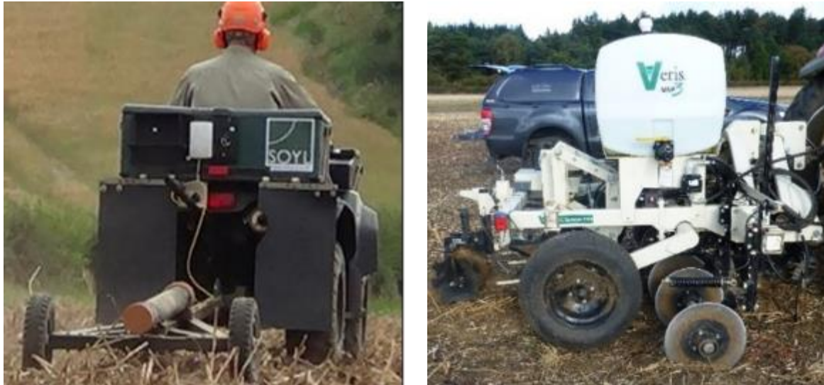
Figure 20. Measuring soil electrical conductivity using a non-contact EMI scanner (left) and a contact Veris MSP3 EC scanner
